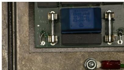
Lay the equipment (still unopened) back onto its back, and then lift off the housing cover. You can now replace the error fuses with new ones. (4 x 20mm 4AT microfuse).
