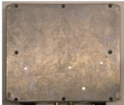
Disconnect the equipment from the power supply. Dismantle the FC 1000 by loosening the four fastening screws (see section 3.1).
